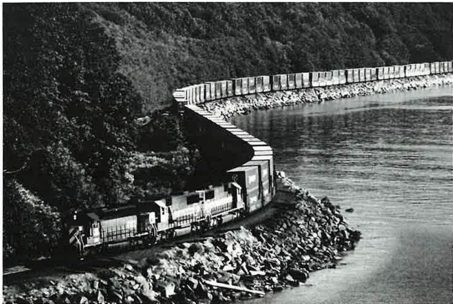
A typical double-stack train can carry 480 twenty-foot equivalent units.
