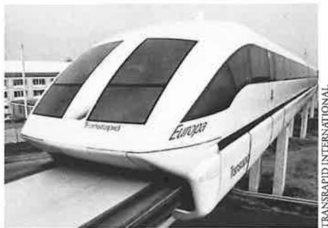
Transrapid 07 prototype revenue vehicle at the Elmsland 32-km (20-mile) test and demonstration site near Lathen, Federal Republic of Germany.
