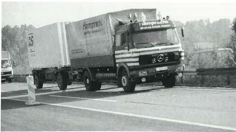
Trucks on European highways are about 20 percent heavier than their U.S. counterparts and often are equipped with single instead of dual wheels.
