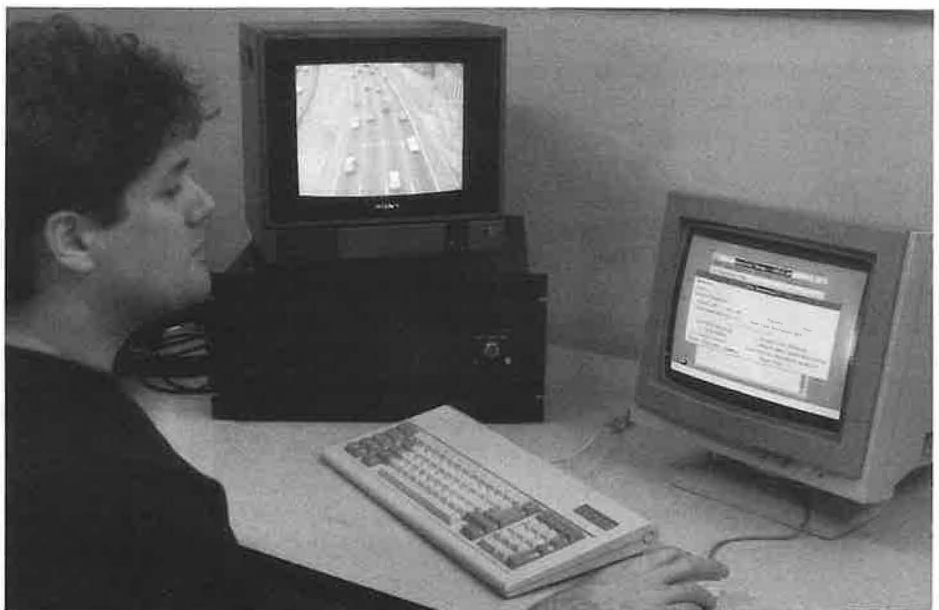
Advanced applications in traffic surveillance and control, such as this video imaging vehicle detection system, could further automate identification of congestion levels, detection of major incidents, and control of traffic signals.
