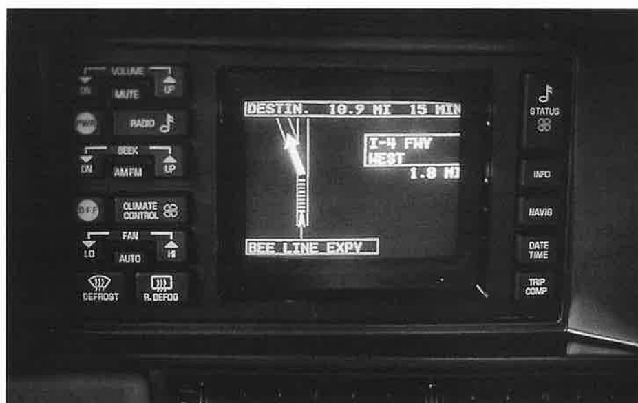
Travelers could receive information from in-vehicle displays on estimated trip duration or alternative routes or modes.
