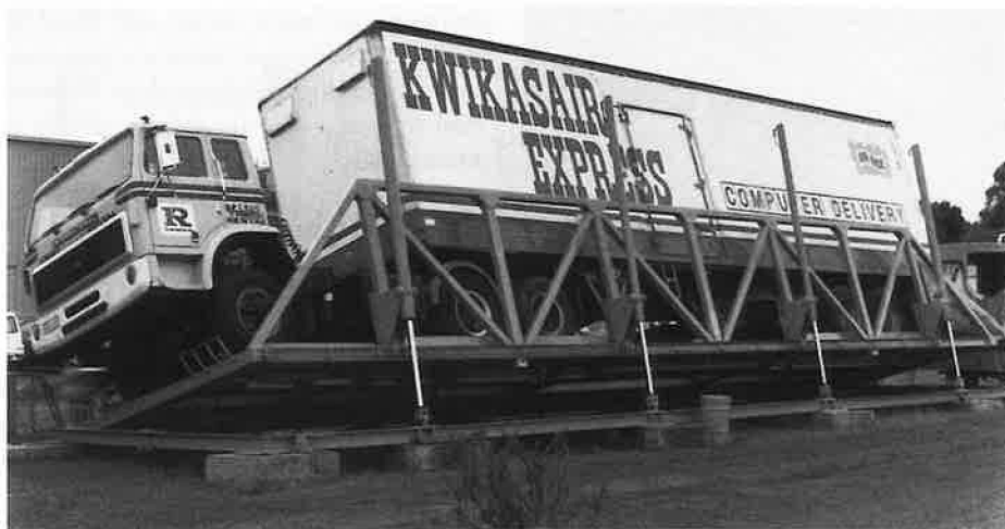
FIGURE 6 ARRB is developing truck rollover warning device using equipment such as tilt-deck, shown here.
