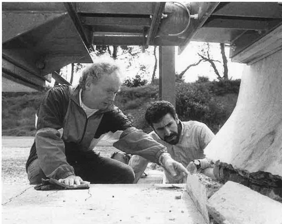
Andrew Scanlon (left), Professor of Civil Engineering and Director of PTI's Transportation Structures Program, and graduate student Abbas Aminmansour examine results of impact testing on concrete barrier.
