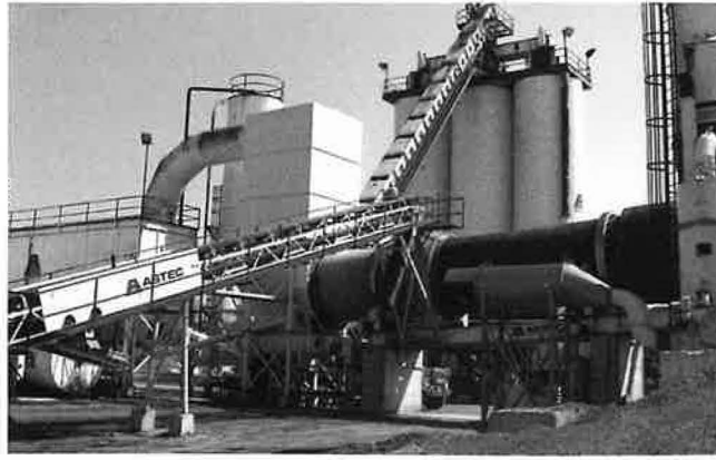
Drum mix plant used to produce SMA for a 1992 U.S. project. Stabilizer has been added at center of drum along conveyor belt.
