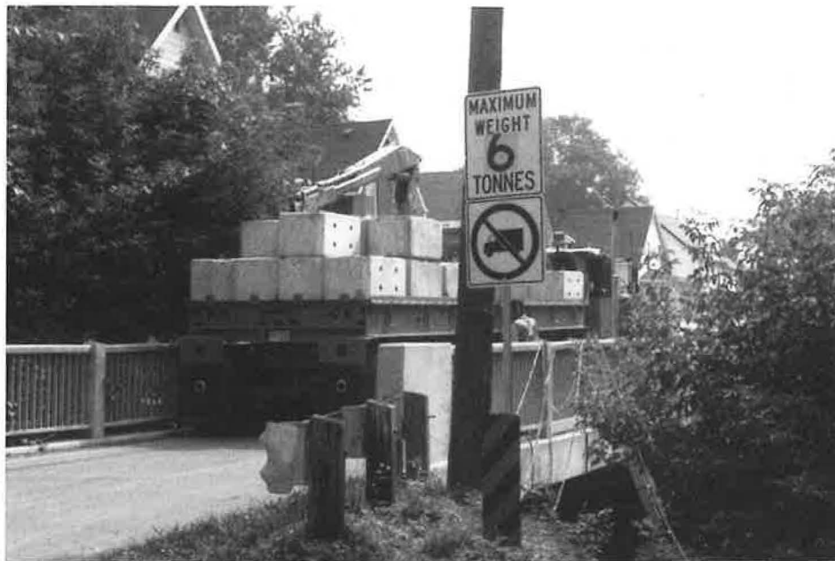
Vehicle conducts proof test on posted bridge to determine validity of restrictions.
