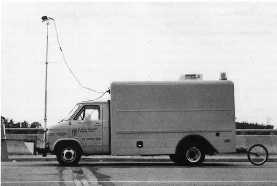
Self-contained prototype vehicle that uses radar and thermography is now part of MTO's bridge management system. Vehicle detects deck deterioration and determines asphalt thickness over concrete and concrete cover over rebar.
