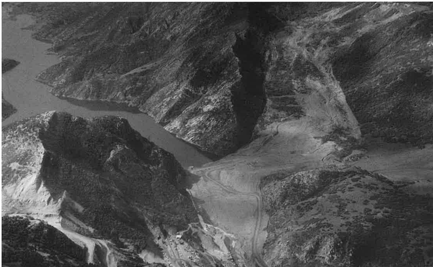
FIGURE 2 Aerial view of April 1983 Thistle debris slide, Utah. Photograph from September 1983 shows Thistle Lake, which was impounded by the landslide, the realignment of the Denver and Rio Grande Western Railroad (lower center), and the large cut for rerouting U.S. Highway 6/50 (extreme lower left).
