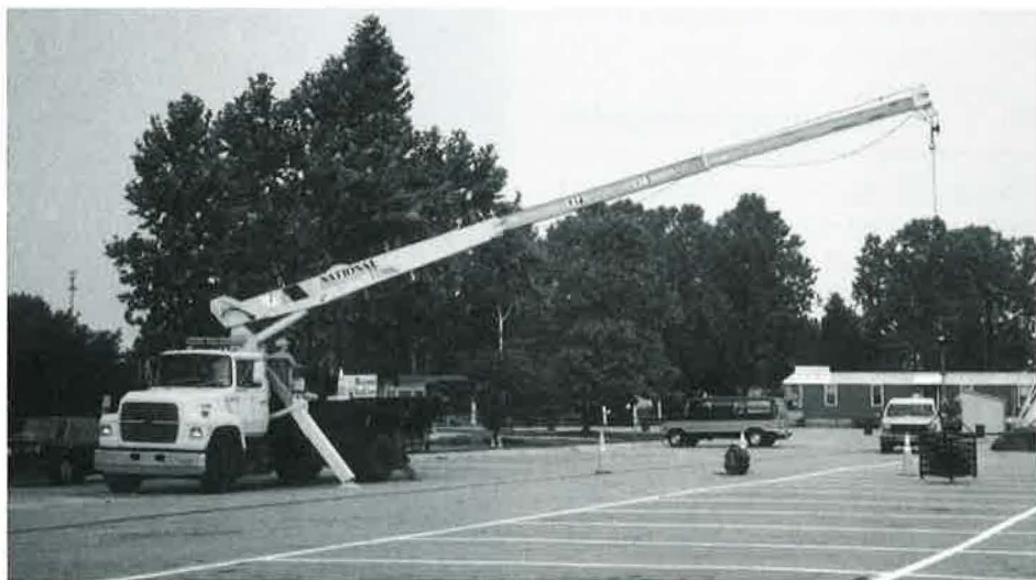
FIGURE 1 NCDOT's sensor-equipped crane during experimental test.
