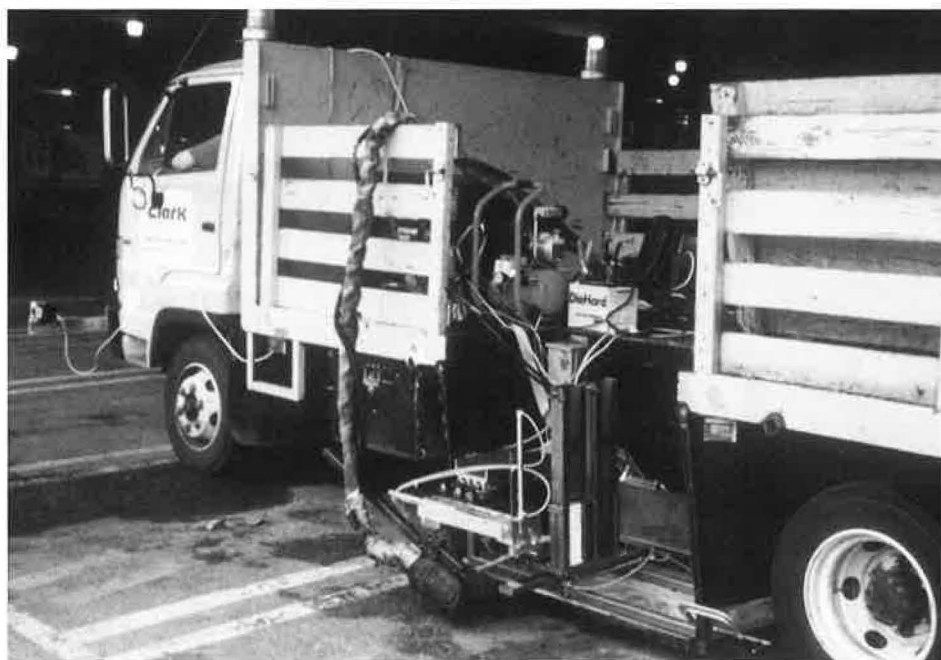
FIGURE 4 Installation of telerobotic raised pavement marker applicator on truck.
