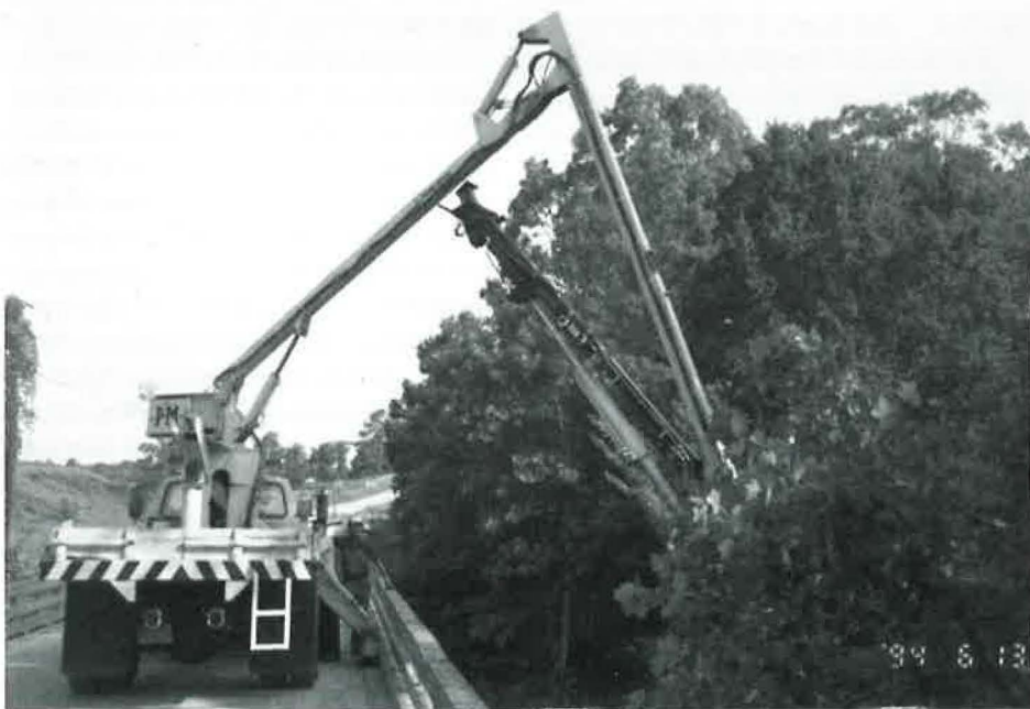
FIGURE 7 Deployment of Robotic Bridge Paint Removal system for field testing.
