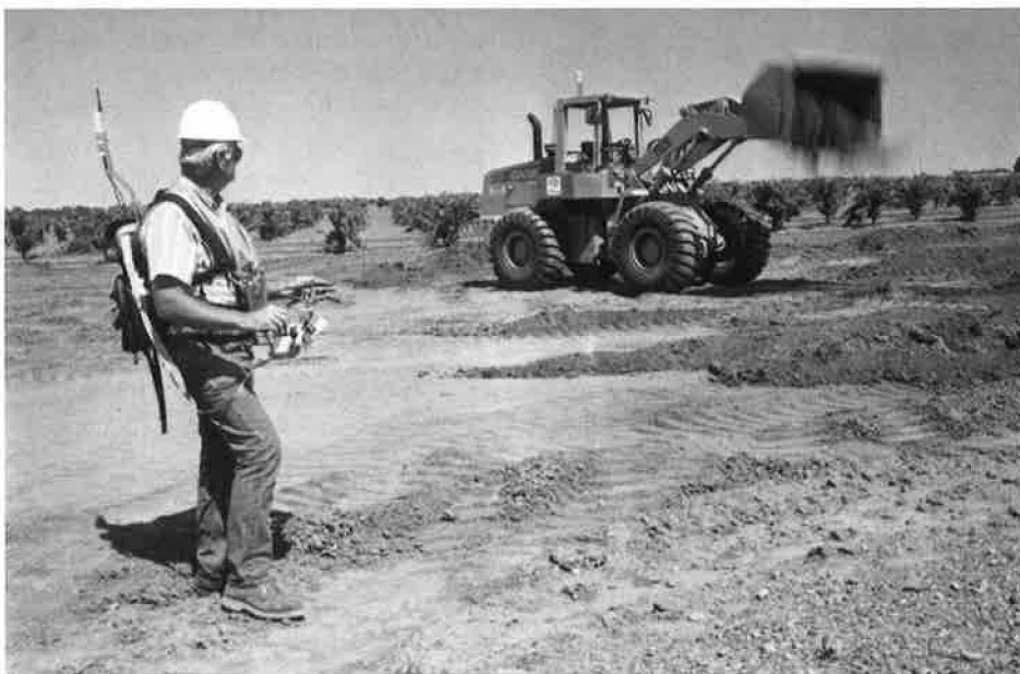
FIGURE 8 Teleoperated and automated maintenance equipment robotics operated from backpack-mounted controller.
