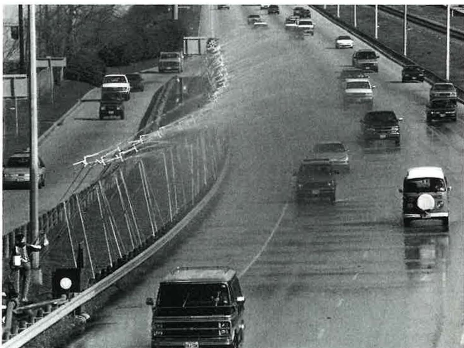
Rainfall simulator designed by Center for Research in Water Resources sprays traffic and road surface on MoPac Expressway in Austin, Texas.
