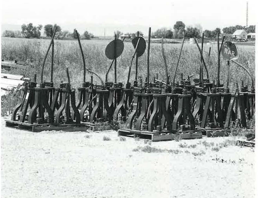
Secondhand rail anchors are sorted, bagged, and loaded for shipment to track-renewal projects (top). Damaged or worn switch stands that have been sorted and unloaded will be rebuilt by a contractor and returned to use in main track (bottom).
