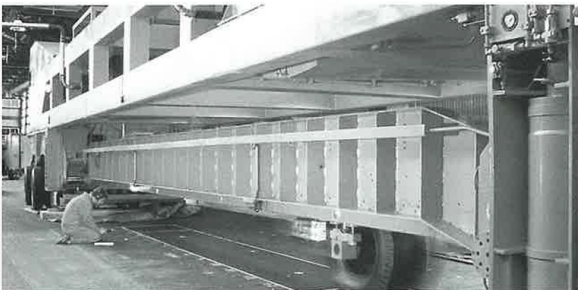
FIGURE 4 Caltrans Heavy Vehicle Simulator tests pavement at Richmond Field Station, University of California, Berkeley.
