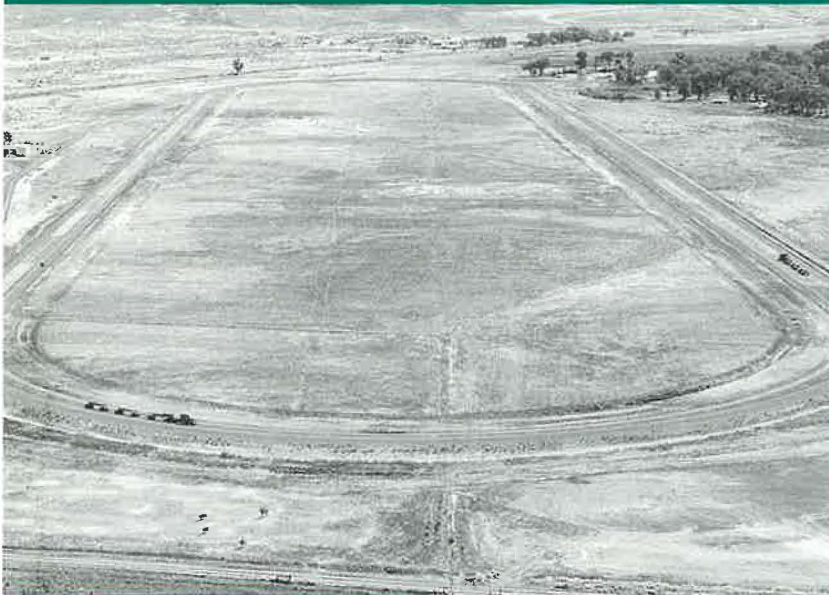
WesTrack, located in the Nevada desert, includes test sections to validate the Superpave system.
