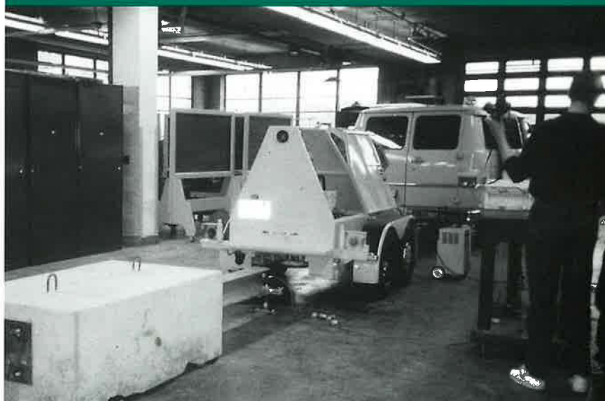
Regional calibration centers allow highway departments to determine if falling weight deflectometers are functioning properly and producing consistent results.
