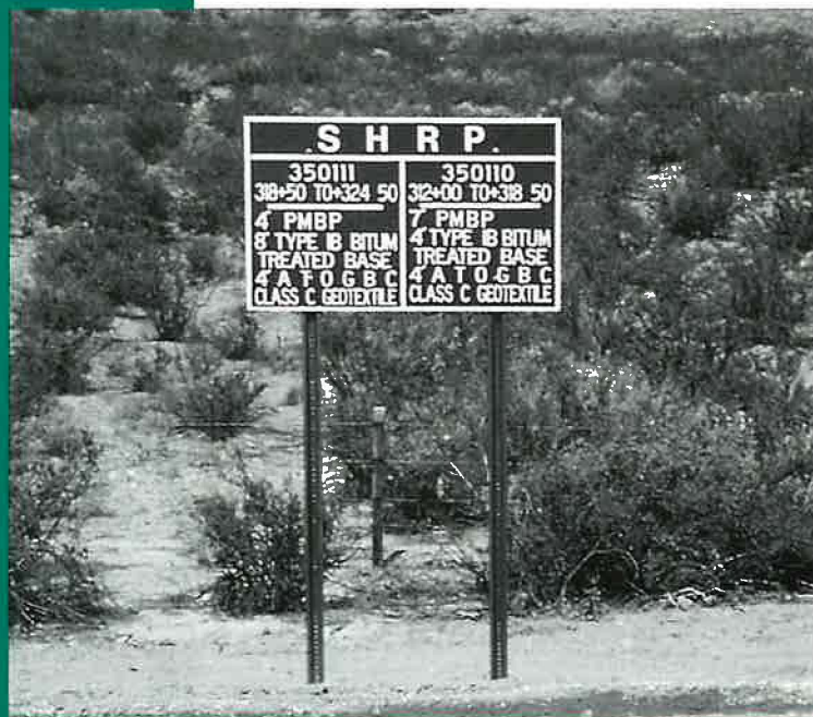
More than 1,000 specific pavement study test sections are located at 200 sites throughout North America.
