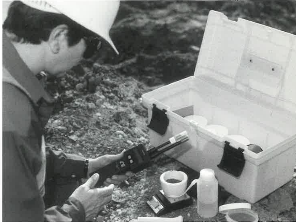
FIGURE 2 Use of soil stabilization kit developed by Texas Transportation Institute and alternative stabilizers, such as low-calcium fly ashes, could save Texas as much as $23 million per year in pavement repair costs.
