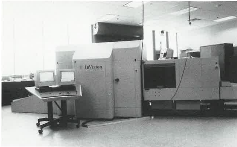
CTX 5000, developed with FAA support, uses transmission X-ray data to acquire an overall map of objects in luggage.
