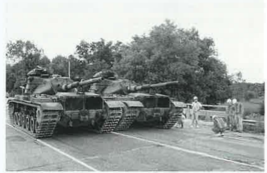
M-60 military tanks were used by the University of Michigan for proof load testing.
