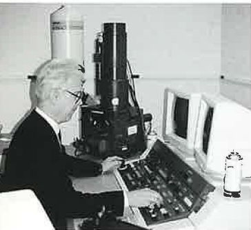
Metallurgist in NTSB materials laboratory examines fragments of material under scanning electron microscope to determine origin and cause of a fracture.
