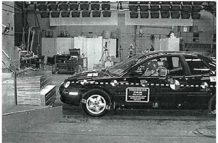
This 40-km-per-hour, 40 percent offset test is part of advanced frontal research in support of improved occupant protection.
