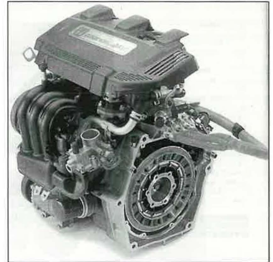
FIGURE 7 Honda Insight high-efficiency engine with integrated electric motor.
