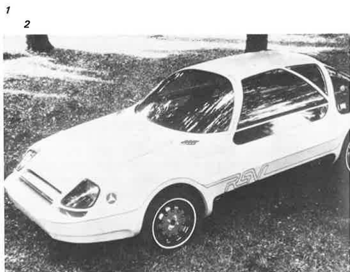
2 Minicar's sporty approach to the RSV emphasizes maximum visibility, gull-wing doors, electronic instrument display, air bag protection, and radar-actuated braking.
