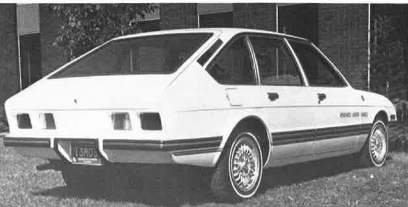
1 Research safety vehicle developed by Calspan and Chrysler is loaded with many features including reinforced structure; soft front end, rear, and interior; run-flat tires; and Inflatabelt restraints. The car weighs 1361 kg (3000 lb).
