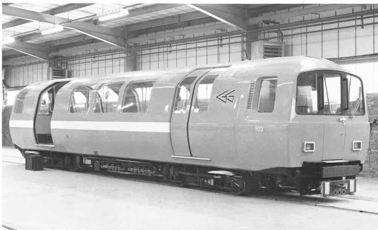
New cars are 12.75 m long, 2.34 m wide, and 2.65 m high. They will be operated at first as two-car trains, and later as three-car trains. They accommodate 36 seated passengers and 56 standees.
