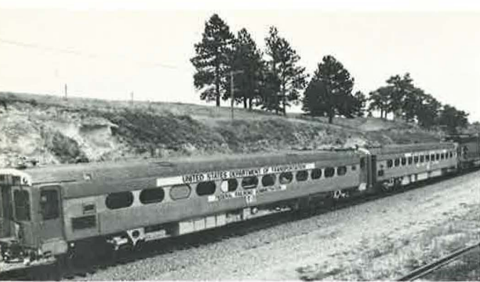
The two-car T1/T3 inspection facility is propelled by a locomotive unit belonging to the railroad that is being inspected. It is equipped with high-intensity halogen lights on the roof and lights mounted underneath the coupler.
