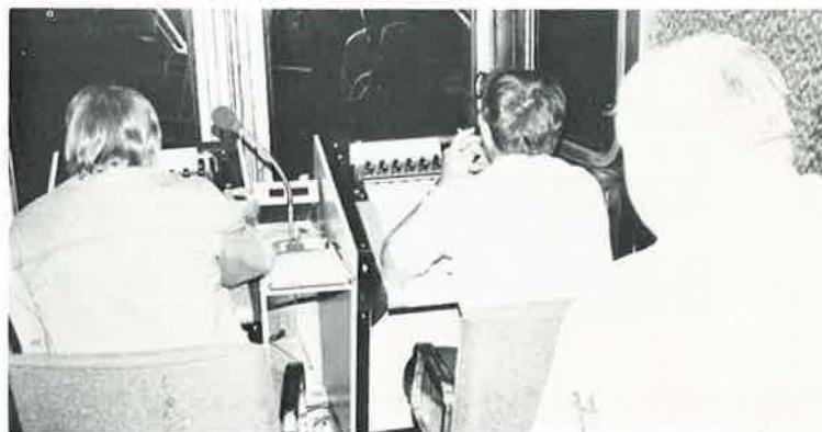
The interior of the T3 observation area includes two eight-channel oscillographs. They are being used here by an FRA inspector and a railroad representative.
