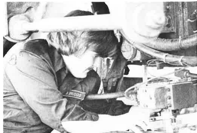
A technician verifies the calibration of the gage-measuring sensor mounted underneath the car.
