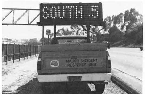
A changeable-message sign truck is stationed on the shoulder of the San Diego Freeway. Electronic signs are programmed with up to five words, and messages can be changed readily to keep motorists up to date on changing conditions.
