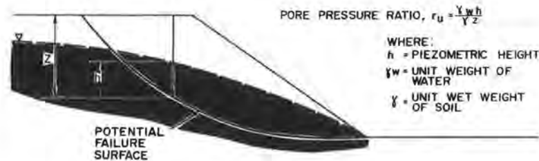
Figure 3. Definition of pore pressure ratio ( r_u ).
