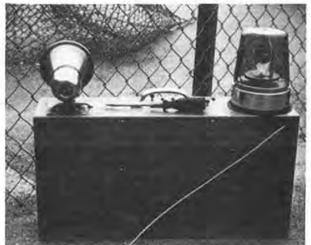
Figure 8. Surface extensometer alarm system.
