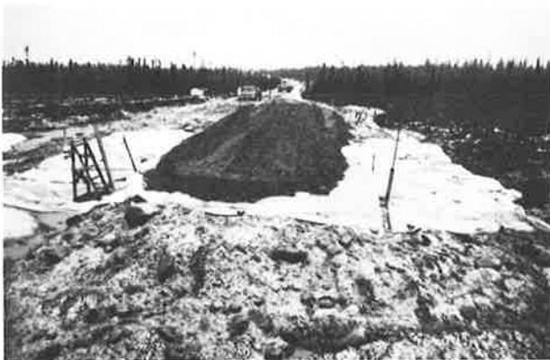
Figure 12. NBR-3 test site: sloughing of slope material.
