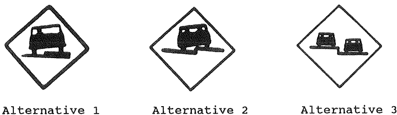
FIGURE 4 Alternatives for Uneven Pavement sign.
