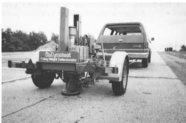
FIGURE 12 Dynatest Falling Weight Deflectometer.
