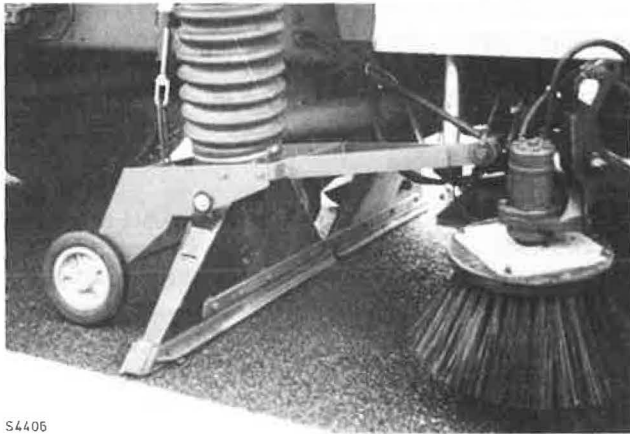
FIGURE 12 Cleaning the surface with an appropriate suction sweeper using a water jet.
