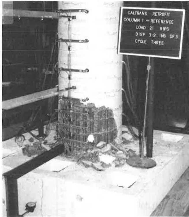
Figure 6: Bond Failure in Column 1
