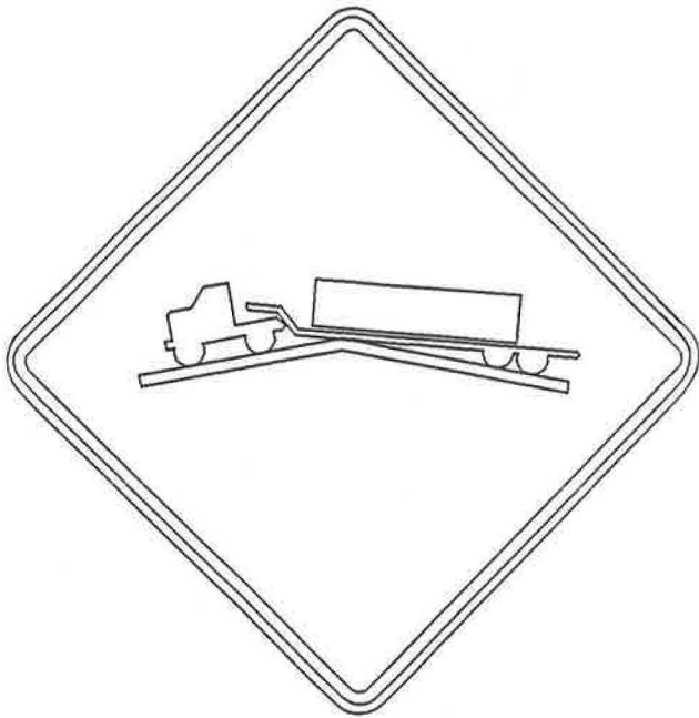
FIGURE 1 Low-clearance-vehicle warning sign proposed by North Carolina Department of Transportation.
