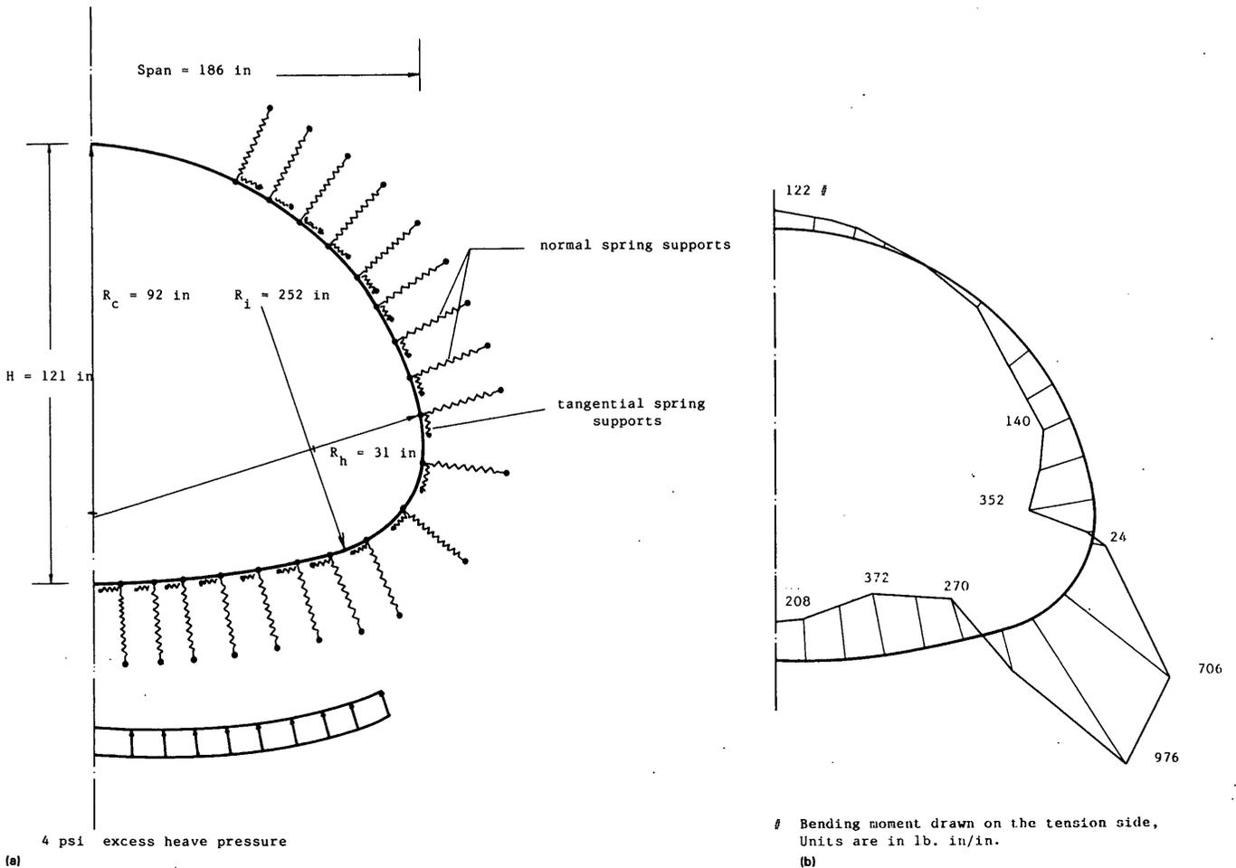
FIGURE 1 (a) Model for conduit analysis; (b) bending moment induced by heave pressure at the invert. Span  $D_H = 186$  in.; rise = 121 in.; radius at crown  $R_c = 92$  in., at invert  $R_i = 252$  in., at haunch  $R_h = 31$  in.; and heave pressure = 4 psi.
