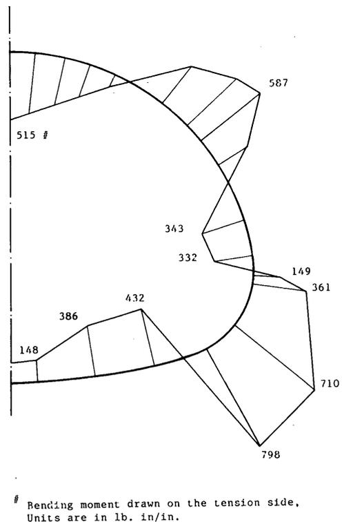
**FIGURE 2** Bending moment induced by loss of soil support (stiffness) at the haunches. Spring supports at haunch reduced by 40 percent. Span  $D_H = 186$  in.; rise = 121 in.; radius at crown  $R_c = 92$  in., at invert  $R_i = 252$  in., at haunch  $R_h = 31$  in.
