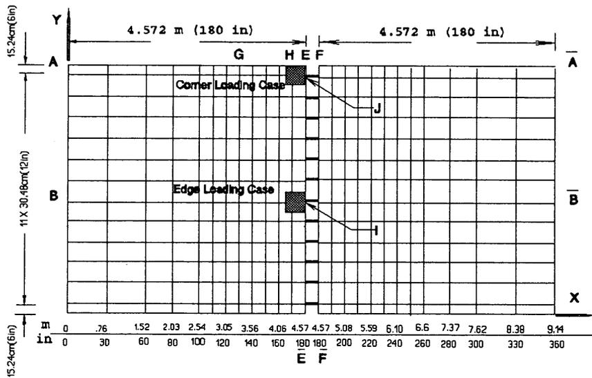
**FIGURE 2 Finite element mesh and two load cases.**
