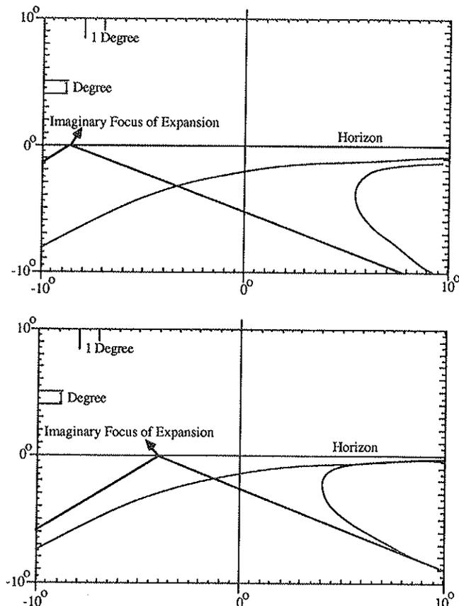
FIGURE 1 Perspective views of typical right curves: top, radius = 200 ft; bottom, radius = 1,000 ft.
