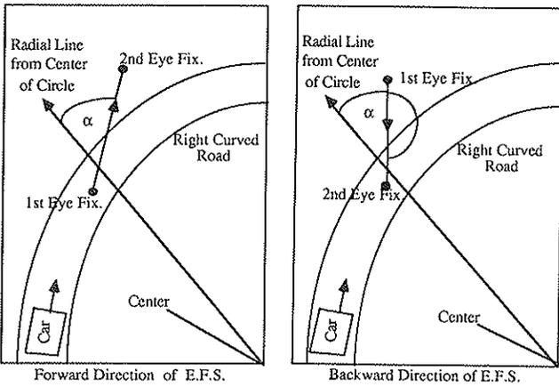
**FIGURE 3** Graphical definition for direction of single EFS: *left*, 0 degrees  $\leq \alpha < 180$  degrees; *right*, 180 degrees  $\leq \alpha < 360$  degrees.
