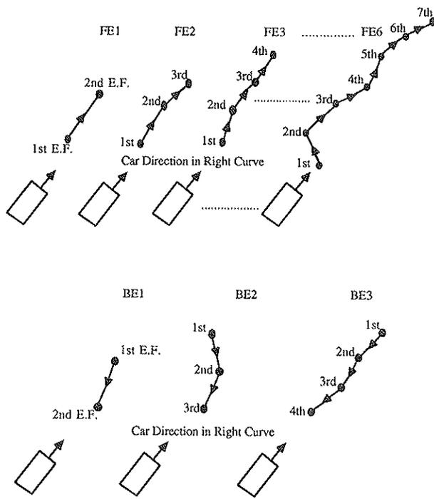
**FIGURE 5** Graphical definitions for forward ending sequences (*top*) and backward ending sequences (*bottom.*)
