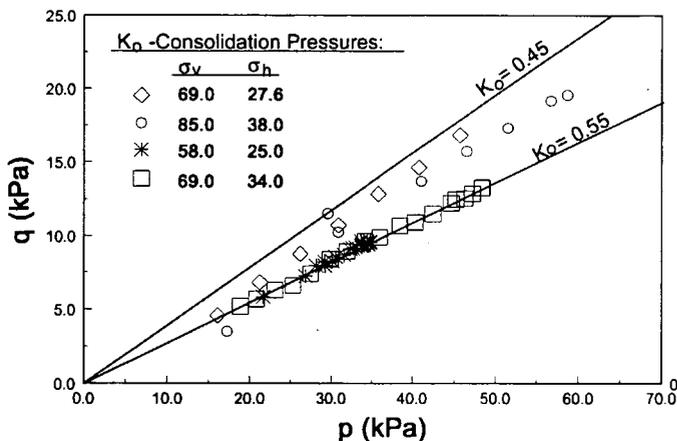
FIGURE 7 Measured  $K_0$  values from CC test [ $\sigma_v$  = vertical consolidation stress,  $\sigma_h$  = horizontal consolidation stress,  $q = (\sigma_v - \sigma_h)/2$ , and  $p = (\sigma_v + \sigma_h)/2$ ].
