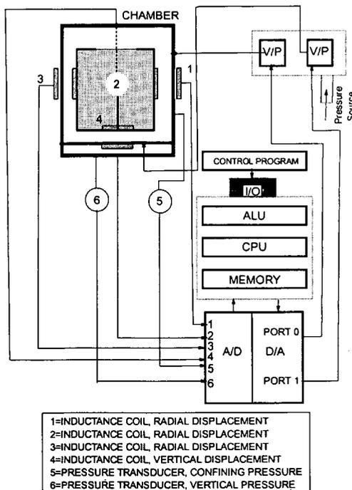
**FIGURE 5** Closed-loop computer control system (ALU = arithmetic logic unit, CPU = central processing unit).
