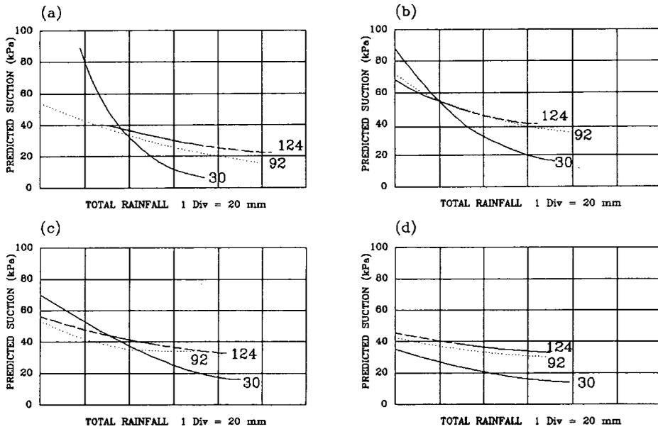
FIGURE 10 Suction reduction prediction curves for all berms: (a) Berm 1, (b) Berm 4, (c) Berm 3, and (d) Berm 2.
