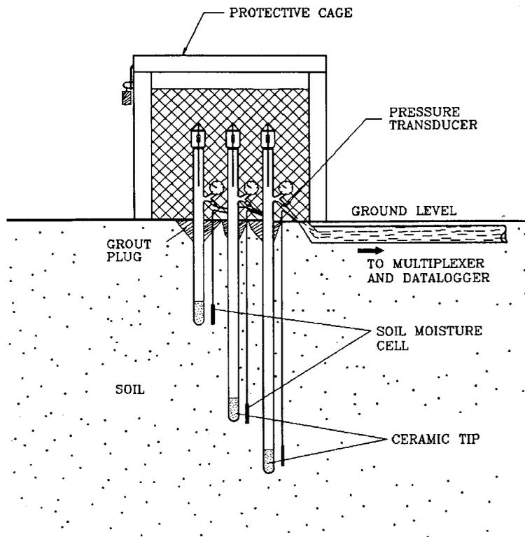
FIGURE 7 Typical instrumentation details for a single location.
