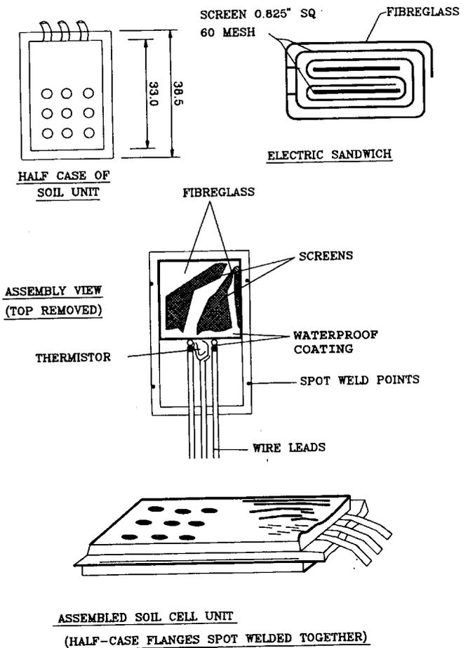
FIGURE 3 Details of the soil moisture cell.
