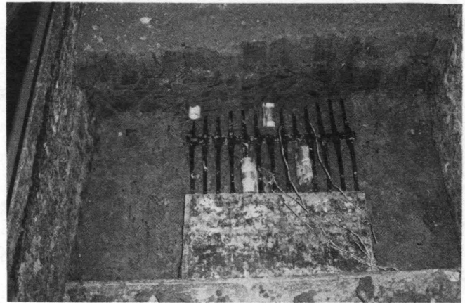
FIGURE 5 Placement of instrumented HDPE geogrid in confined extension test.
