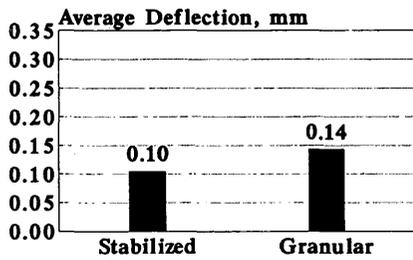
**FIGURE 4** Effect of base (stabilized versus granular deflections.)
