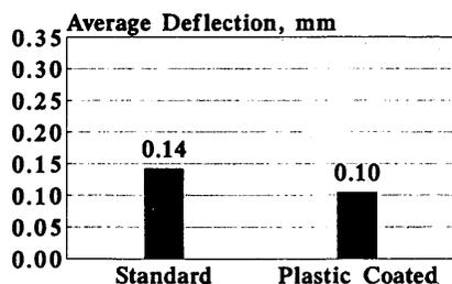
FIGURE 9 Effect of dowels (standard versus plastic coated).
