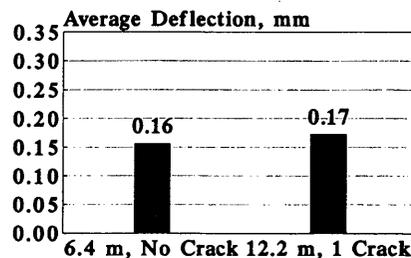
FIGURE 12 Effect of joint spacing (6.4 m, no crack versus 12.2 m, one crack on granular base).
