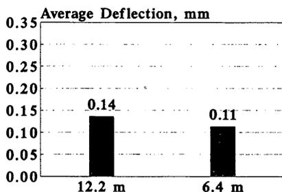
FIGURE 10 Effect of joint spacing (12.2 versus 6.4 m).
