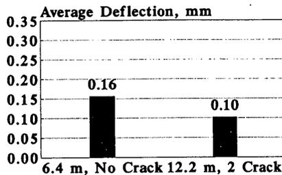
FIGURE 14 Effect of joint spacing (6.4 m, no crack versus 12.2 m, two cracks on granular base).
