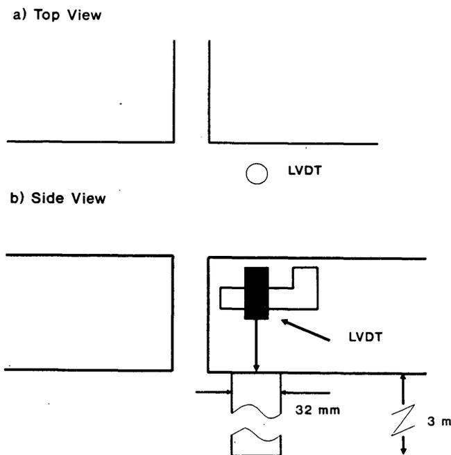
FIGURE 1 Placement of LVDT on pavement.
