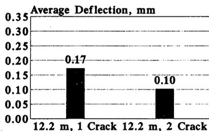
FIGURE 11 Effect of joint spacing (12.2 m, one crack versus 12.2 m, two cracks on granular base).
