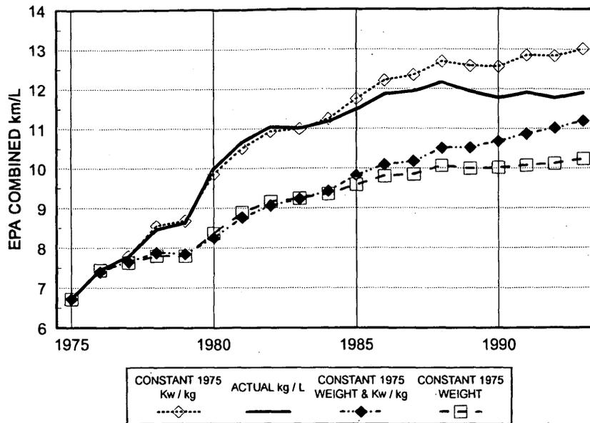
FIGURE 9 Effects of weight and horsepower on passenger-car fuel economy.
