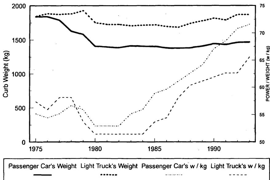
FIGURE 8 Passenger-car and light-truck weight and performance.
