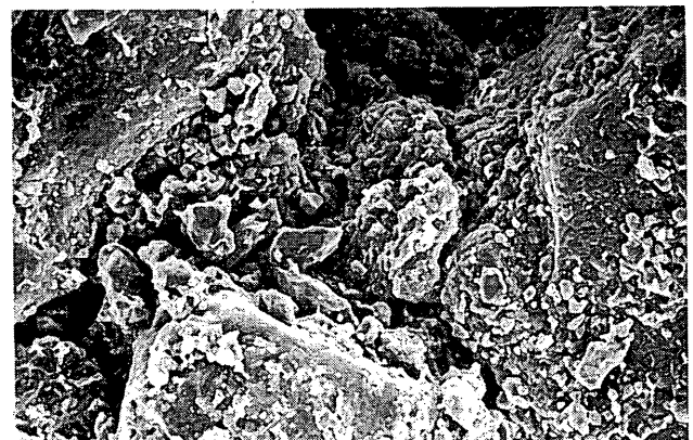
FIGURE 6 SEM image of stabilized caliche ( \times 370 ).
