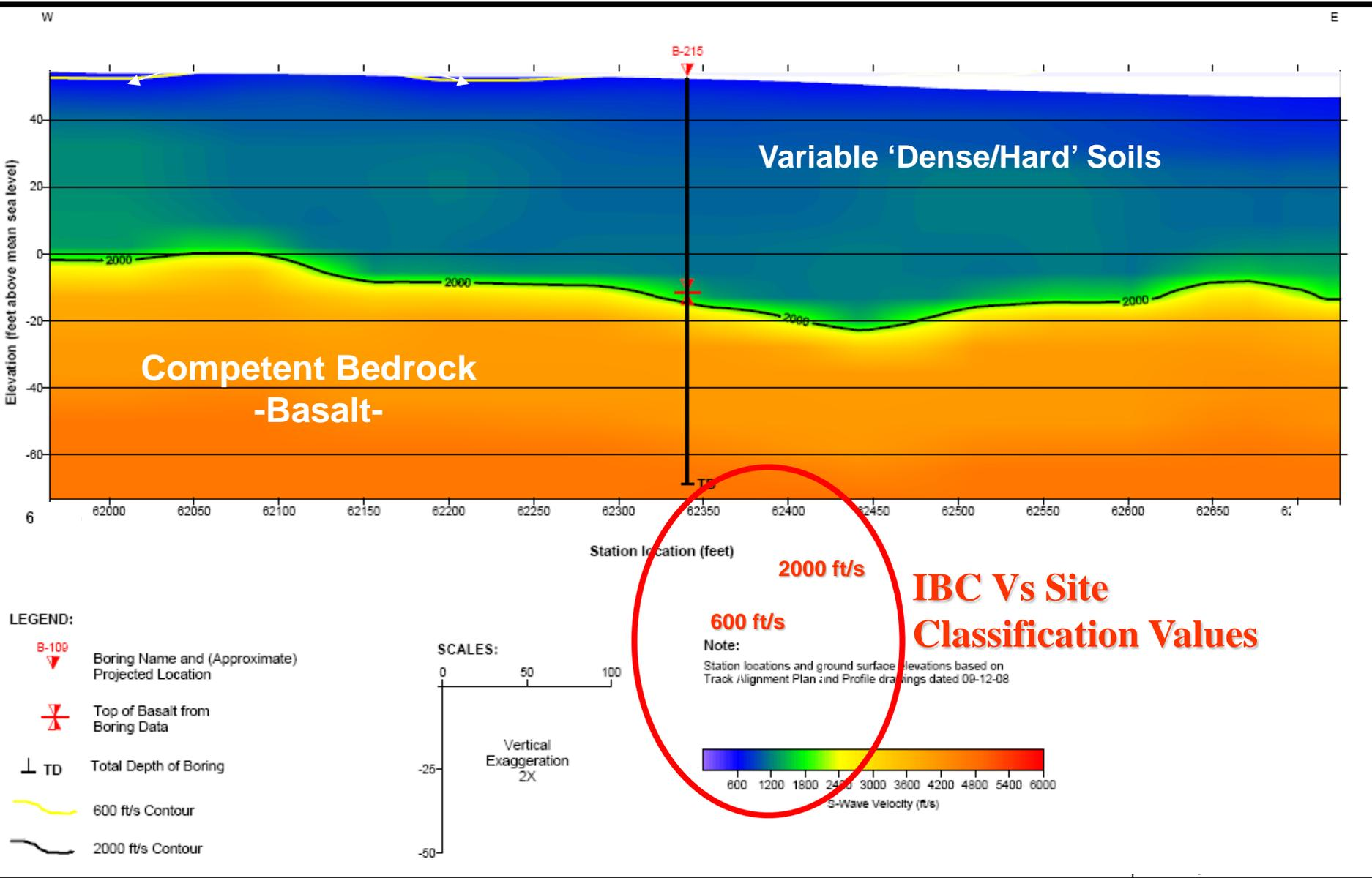
**TEST LINE 1 → Finalized Vs Section with Seismic Interpretation and Geology**
