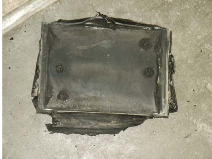
Figure C-11 Trial Bearing after Testing at Excessive Frequency and Rotation Amplitude.
