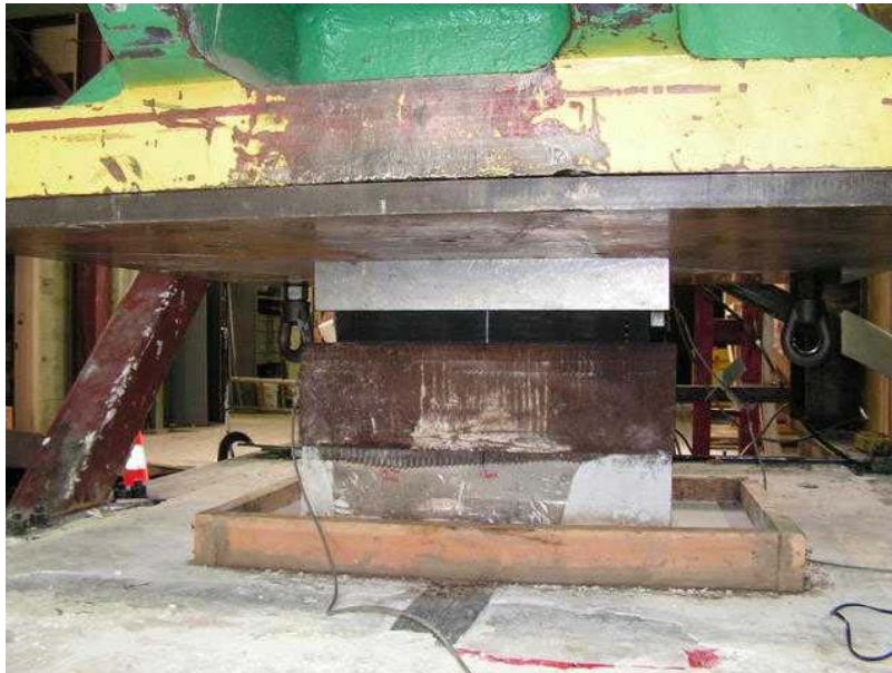
Figure C-13 Axial Test Setup Photo
