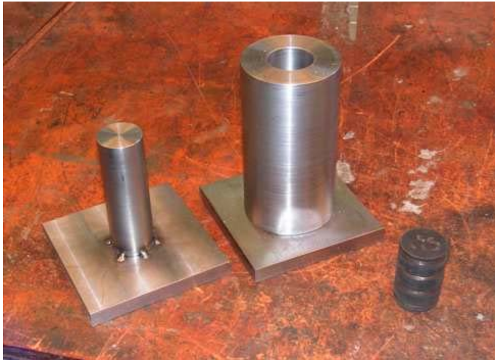
Figure C-20 Bulk Modulus Test Rig and Sample
