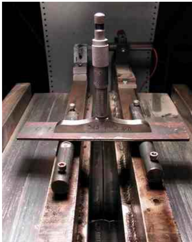
Figure C-10 Depth Gauge Shown Measuring Bulge
