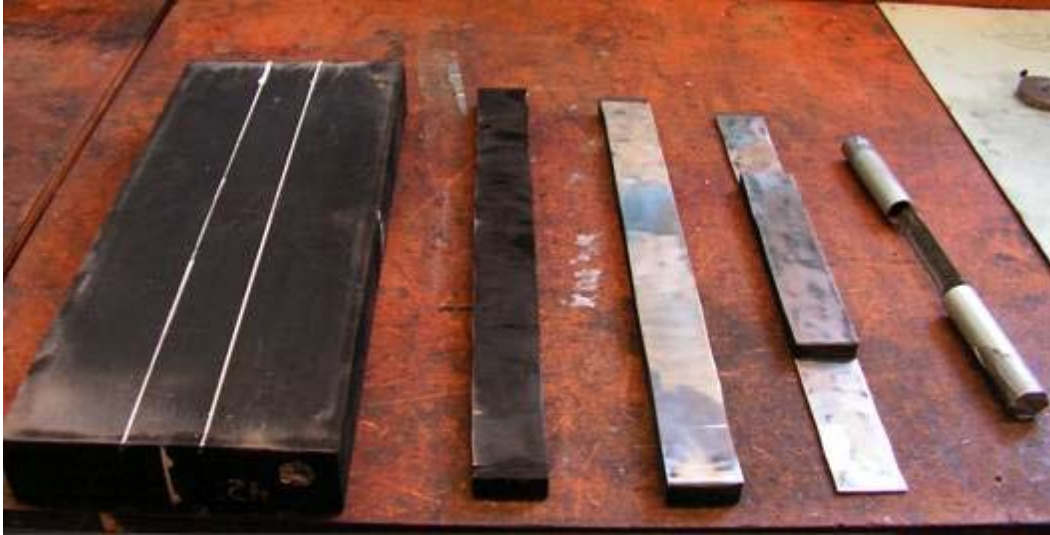
Figure C-18 Shear test specimen in various stages of production. The knife for peeling off rubber is also shown far right.
