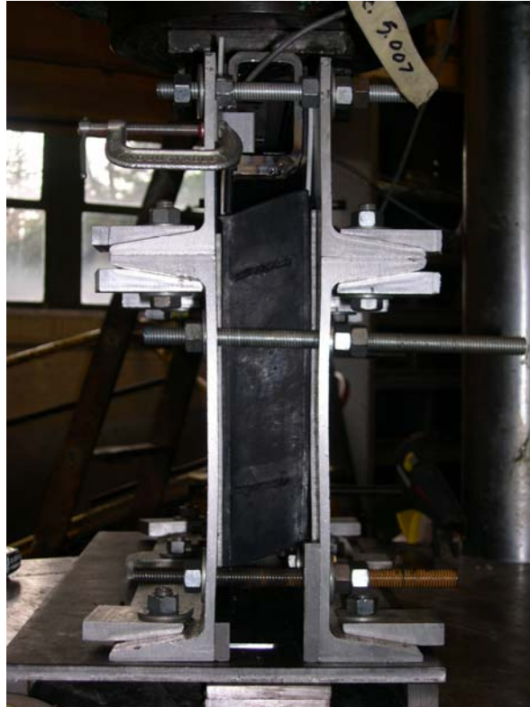
Figure C-16 Torsion Box with Bearing under Load
