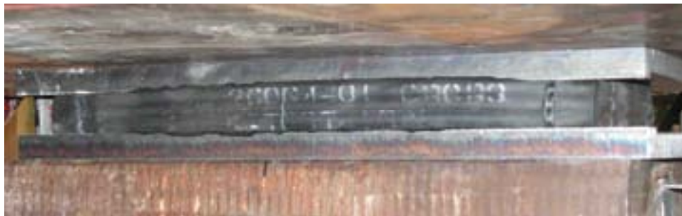
Figure D-6. Bearing Slips out of Tapered Plates during Test
