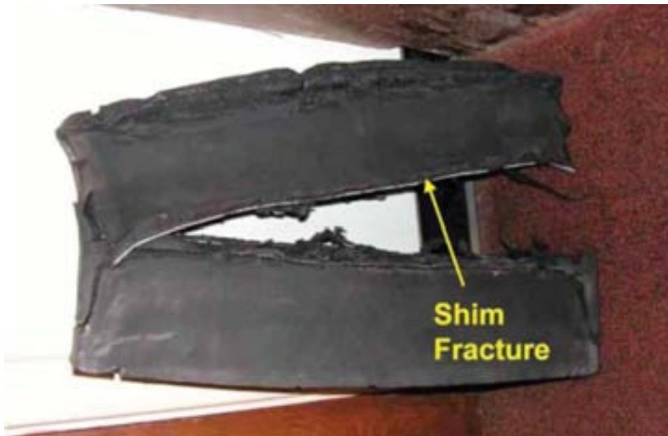
b) Bearing After Removal from Test Frame
