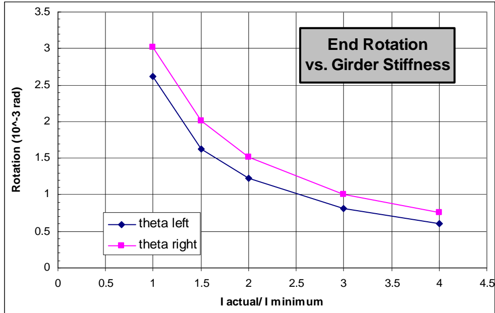
Figure F.33. Effect of Girder Stiffness on Rotation Angle.
