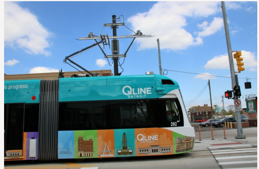
Detroit Streetcar Pantograph Charging at Station (open air)
