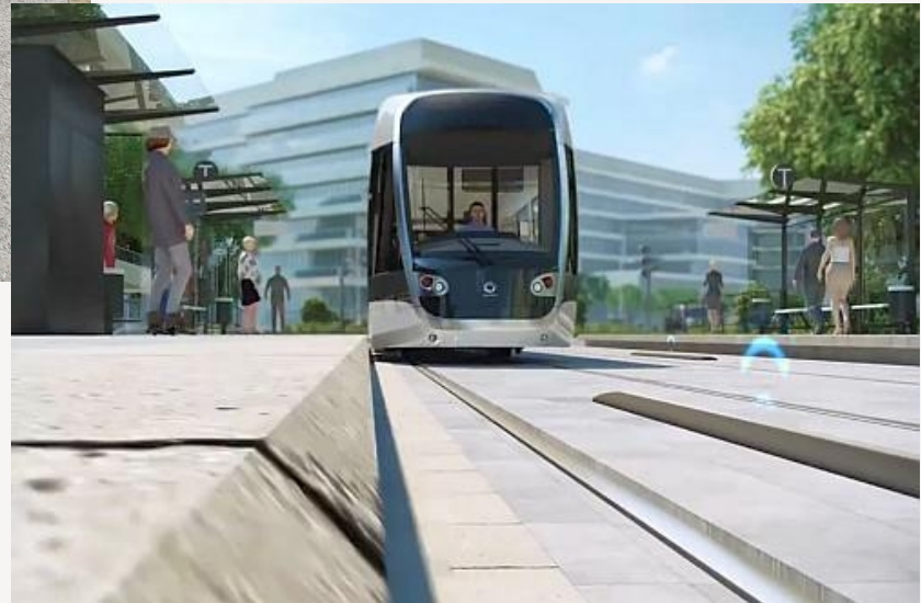
Rio de Janeiro Ground Level Charging Point at Station (SRS)
