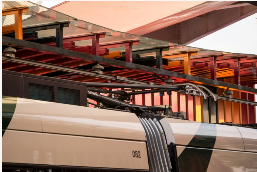
Kaoshiung Pantograph Charging at Station (under canopy)
