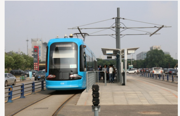
Shenyang, China Pantograph Charging at Station (open air)
