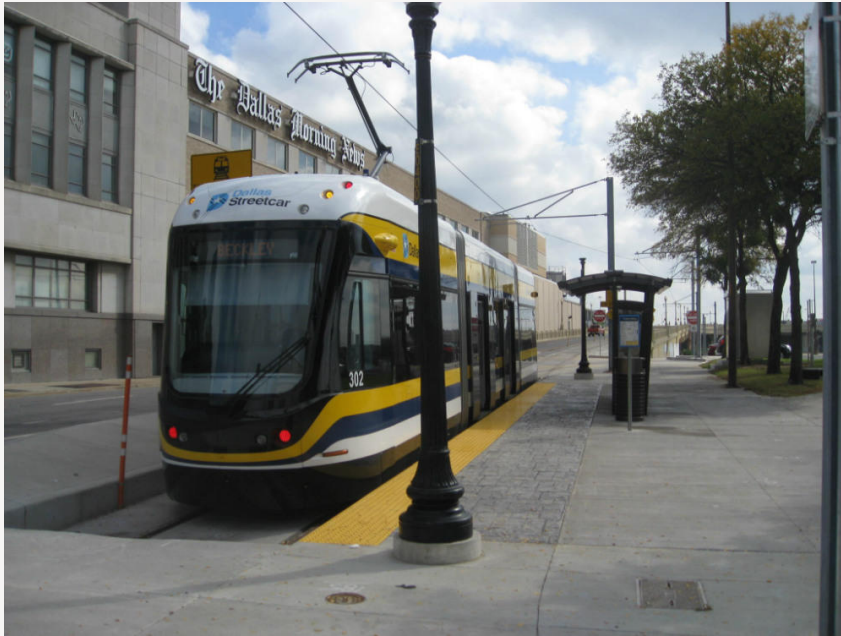
Dallas Oak Cliff Streetcar Pantograph Charging at Station (under OCS)
