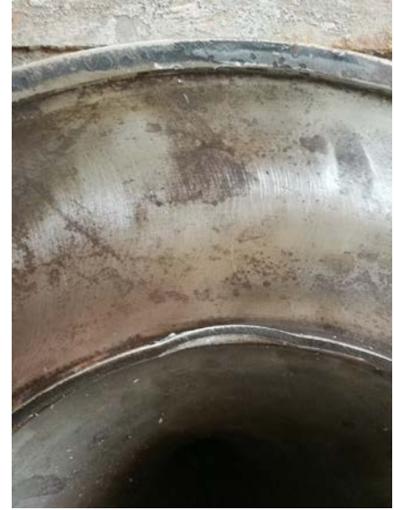
Fig. 34(a). Hysteresis loops when imposed lateral displacement has surpassed the design deformation capacity of a VC2 specimen; higher resistance presents when the pin is pushed to the side and touches the wall of the VGT; (b) the over-powered push left an indentation on the corner between the V tube and top pad while the hysteresis behavior is still on-going.
