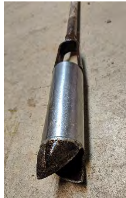
Figure 20 Manual soil core used to collect soil samples from the bottom of the boreholes
